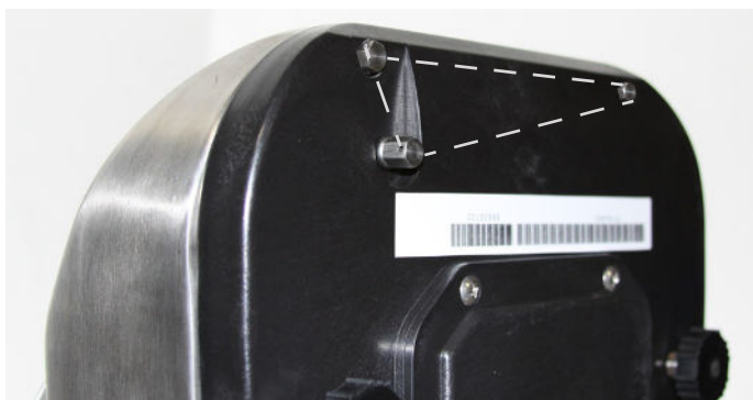
Figure 3-2. Legal for trade seal; cable passes through three bolts
